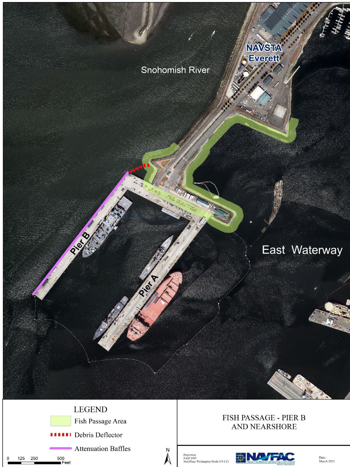
Figure 2-41. Baffle mitigation - Fish passage through Pier B.
